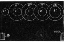
or the amount of weight required to move them? A. Disregarding friction, the power and weight are to each other in the inverse ratio of the distances passed over by each in the same time. Is there any rule for calculating the power of coil springs? A. The power of a coiled spring is the product of the force with which it tends to unwind multiplied by the distance passed over by the point of application of the force in a given
