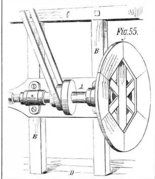
firmly fixed to the joists, C, and to the flooring at D, right over and upon the joists supporting the flooring, or else upon beams provided for the purpose. By this means the work may, if the lathe head is fixed midway upon the posts, B B, be as large as the space between the ceiling and the flooring will admit, a movable tripod rest, such as shown in Fig. 47, being employed for a tool rest.
