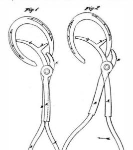
ened or spread. To bend the shoe, the long jaw, C, is placed within the shoe, with the end of the arm, D, resting against the arm of the shoe to be drawn inward or bent, and with the short jaw, E, resting against the outer corner of the heel of the said arm of the shoe. Then, by moving the han dles toward the heel of the other arm of the shoe, the said shoe will be bent or contracted.
