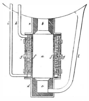
water. The molten metal is conducted in the ordinary manner by a conduit, l, which terminates at the lower portion of the lower transion, e. In the same way as the cooling can be regulated by the length of the water circulation, so can its intensity be varied by regulating the temperature of the
