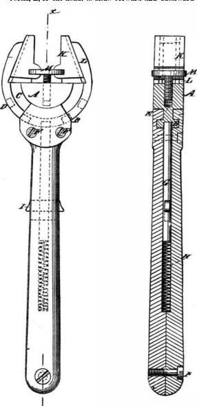
to be adjustable for different sized nuts. The disk-headed crew, M, is notched in the jaws and screwed'in the head so as to work the jaws backward and forward.
