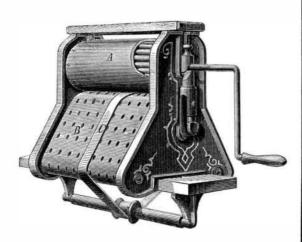
to the rolls while the water may be used much hotter than usual. The rubber conforms to the uneven thicknesses of the clothing. The machine is designed to be used in an ordinary washtub.
