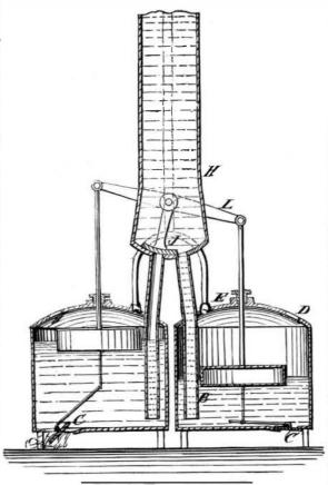
rod. The valves, at C, are so connected to the floats that, when they are raised by the water to the required hight, the floats open them to let the water escape and reverse the machine. By the filling of the cylinders with water the air is forced out through outlet, E, into the receiver; and by the escape of the water the cylinders fill with air again, to be again expelled into the receiver. This device was patented October 24, 1876, through the Scientific American Patent.
