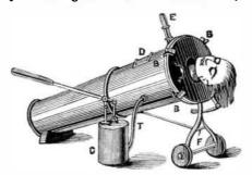
by the descent of the diaphragm. All returns to the former position when the lever is raised again. These complete respiratory movements may be repeated fifteen to eighteen times in a minute, as in a living man.
