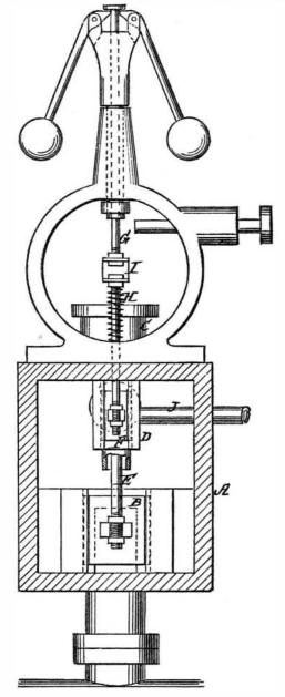
valve, B; and when the balls fall, it will admit steam to the lower end and raise the valve, B. The spring, H, on the rod of valve, F, balances the weight of the valve. The valve, F, can be set for high or low speed by the adjustable coupling, I. J is the exhaust pipe for engine, D. It is pro-
