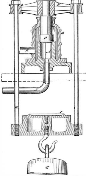
be used to any given pressure by simply adding weights up to the required amount.
