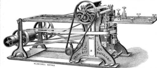
We have sold 160 of these planers within the last 20 months, all of which are giving good satisfaction. We build two sizes, to surface 20 and 24 in. wide, and tongue and groove from 14 to 18 in. wide, and surface from 14 to 6 in. thick, at prices varying from \$250 to \$325. For further information, address
