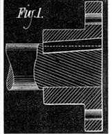
lasting hills. I know I never heard of it before. Fig. 1 shows the method The key seats in both shaft and hub draft the same way, and the key is consequently straight. If the fit is simply neat, the thing is firmly locked. It applies especially to bevel gearing in millwork, which must back up against something; and in many cases, finding no shoulder on the shaft or convenient box near, the firmness of the hub on the shaft depends on the key
