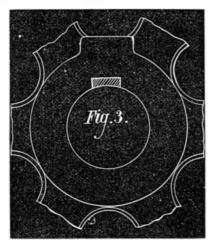
millwrights of the Northwest. The shops up there plane their keys out concave, from a steel strip. They are then cut off, and a little draft given to them. They are tempered blue. The circle of the key should be a trifle smaller than the shaft.'
