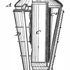
the manufacturers, were the boiler to become red hot, the water would be forced out of it into the receivers, and cannot return again until it has cooled. Though the air valves are self-regulating, and are acted upon by the force of combustion, they can be manipulated by hand if desired, by simply sliding the weight on the arm of the lever, which will open or close the valves, as may be desired.
