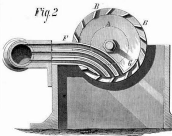
only a greater impetus but, it is claimed, a very high degree of power, considering the pressure and the size of the stream used. Although adapted to all purposes where water is used as a motive power, this invention is more particularly designed for use where the supply of water is limited or variable; and this is believed to be a desideratum, as streams
