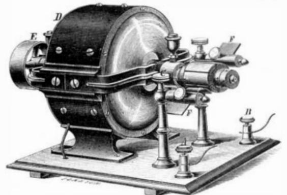
There is, besides, a new and ingenious pole charger which prevents the currents being changed during periods of rest, so that no preliminary examination of the currents is necessary before at once setting the apparatus in operation.
