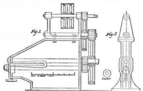
different thicknesses of iron. The two small gear wheels are made of wrought iron, and the other four of cast iron. We run the cutters at about seven turns per minute.
