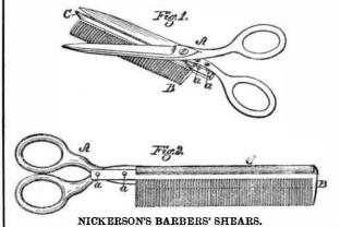
shears, and B is a straight hair comb, arranged outside of and parallel with one of the shear blades, and secured thereto at the inner end by two screw studs, a; and C is a guard
