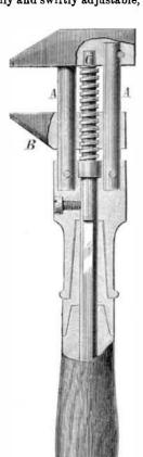
strength and at the same time lightness. It is made of steel; but it is claimed that, owing to its construction and the small amount of metal therein employed, it is no more costly than an iron wrench of common form. It can be produced, we are informed, by special machinery, so that the corresponding parts of any number of wrenches of the same size may be interchangeable.
