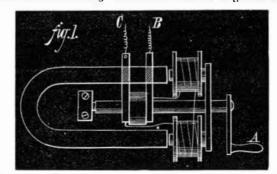
By turning the crank, A, sparks can be obtained either at B or C. These sparks can be obtained at the free or open end of a conductor, by proper connection.
