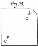
shown in Fig. 197; it is made of sheet iron about one sixteenth of an inch thick, the outline being carefully marked out and filed up nestly, the corner, A, being made of the necessary sweep, and the hole, B, being used to hang the gage up by. It is well to have an assortment of such gages for use in lining out, as well as for use as guides to the machinist in cut-
