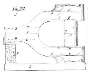
the case, the work is reasonably near to being true, we pro ceed as follows: Placing the double eye upon the marking off table, as shown in Fig. 192, we block up the stem end with the pieces of wood, B, so that the horizontal faces of the work will stand about true with the surface of the table, the manner of testing the same being shown in Fig. 193, A representing the marking-off table, and B the scribing block, with the needle placed so that the point of the
