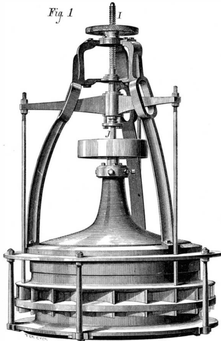
WALTON'S TURBINE WATER WHEEL.
