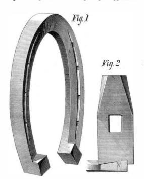
hoof. This peculiar construction is obtained by means of a specially devised swage, the use of which will be understood from the following description.
