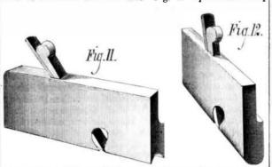
near the front end, are now supplied, and are very useful for cutting out half checks that are not cut right across the stuff.
