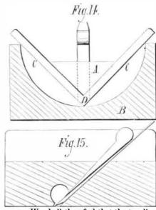
of the groove. We shall thus find that the two lines struck will be at a right angle to each other, the two lines, A A, meeting at the point, a, being at a right angle. The two side faces, C C, of the plane in Fig. 14 are made to stand at a right angle to each other; and while the plane is in position (as shown in Fig. 14) to bear against the corners of the core box, a semicircle (the apex of the plane, D, in Fig. 14)
