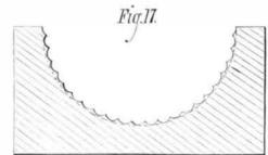
away as much of the stuff as possible before employing it, the work appearing as shown in Fig. 17. These planes have one disadvantage. They are apt to abrade the corners of the work; hence great care should be exercised in their use, and care must also be taken that the extreme point of the plane iron stands just at the apex of the angle of the body of the plane; for if it be in advance or not up to it, the work will not be semicircular.
