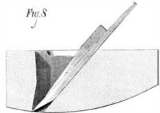
hollow sweeps. This tool is sometimes made adjustable by means of a piece dovetailed in the front end of the plane, as shown in Fig. 9, at A; which, by being lowered, alters the sweep and finally converts it from a convex to a concave. There is now, however, in the market a compass plane, the body of which is made of malleable iron with a sole made of
