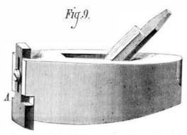
a blade of spring steel, which, by the operation of two screws, can be set to any curvature, either concave or convex, within the capacity of the instrument.
