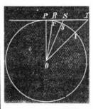
wherein the circle represents a section of the earth through its center, O. PI is the horizon of the point, P, and Rr, Ss, and Ii are hights from which the point, P, can be seen at different distances, Pr. Ps. and Pi. Without going into any mathematical demonstration, it is clear that the hights Rr, Ss, and Ii increase in a far greater ratio than the distances, Pr, Ps, and Pi; but in or-
