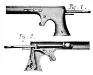
piston rod is a shoulder which, when the rod is drawn back against the spring, C, which bears against disk, A, catches on the handle plate, as shown in Fig. 2. The marble is prevented from rolling out when the piston is aimed downward by the side spring, D. By pressing on the trigger the piston rod is raised so that its shoulder no longer engages with the handle plate, when it is pushed forward by the spring, C, thus throwing out the marble.
