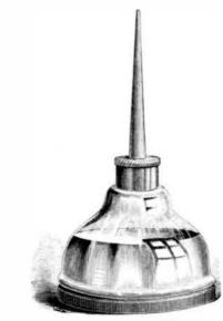
bottom and nozzle are of metal, the former attached around a bead and fastened by cement introduced inside, so as io form a neat and strong joint. The nozzle is a solid, durable piece of Britannia metal, easily straightened if bent, and attached to the can by a screw thread on the glass. The glass is thick and amply strong to resist breakage by any ordinary fall, and it is easily cleansed, and of course it is not subject to corresion
