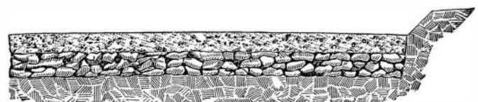
Fig. 5.—ROAD WITH RUBBLE FOUNDATION.
