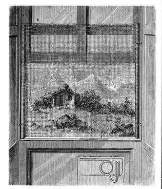
These rollers, about which the cloth is wound so as to adapt it to the width of the window, are held in place by two brass wire clasps, arranged one on each side, and constructed as represented in the sectional view below. On large windows four such clasps would be used. The shanks of the clasps are inserted in closely fitting metal sockets, which last can be easily placed in the window casing by the aid of a gimlet or bradawl. The device is exceedingly simple and very easily adjusted.
