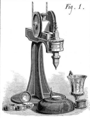
Two tool stocks, A, are arranged side by side in the hollow revolving mandrel, B, so as to slide up and down freely while being rotated. At C are levers suspended by hangers from the pulley, D, which turns the mandrel. These levers are each connected at one end with a tool stock, and at the other embrace the cam ring, E, which is within the casing. As the pulley revolves, the tool stocks are caused to move up and
