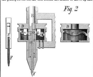
down, so that the tools, F, have a reciprocating as well as a rotary motion. The mandrel is mounted in a bearing at- the present device holds the pipe tached to a stand, and has guide pulleys, as shown, for leading the belt from above to the horizontal pulley. The engraving tools are easily fitted into and removed from the stock, so that they may be changed in accordance with the kind of work to be executed.
