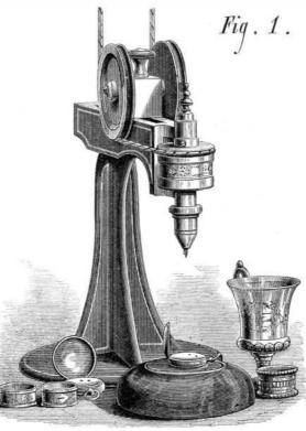
Two tool stocks, A, are arranged side by side in the hollow revolving mandrel, B, so as to slide up and down freely while being rotated. At C are levers suspended by hangers from the pulley, D, which turns the mandrel. These levers are each connected at one end with a tool stock, and at the other embrace the cam ring, E, which is within the casing. As the pulley revolves, the tool stocks are caused to move up and
