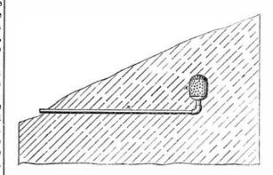
The engraving herewith given shows a section of a side hill or prairie roll, with the device for collecting water in position.
