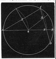
then from center, A, at distance, A C, cut off A H, equal to A C. Draw C D through H. The rest explains itself. A C is the side of an inscribed trigon, C D is the side of a square, D E the side of a hexagon, A I the side of a heptagon, O E the side of an octagon, D B the side of a dodecagon.
