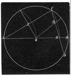
then from center, A, at distance, A C, cut off A H, equal to A C. Draw C D through H. The rest explains itself. A C is the side of an inscribed trigon, C D is the side of a square, D E the side of a hexagon, A I the side of a heptagon, OE the side of an octagon, D B the side of a do-
