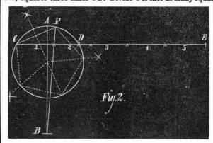
parts as the required polygon has sides. Draw B T, cutting C E, in the first point of section and touching the circle in F. Draw C F, which is the side required.
