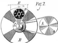
gether by friction gearing. The pulley, E, which, together ith two others the disk can be taken out and replaced by another, like the slides of a magic lantern, while the other parts of the apparatus may remain in undisturbed connection with the lantern.
