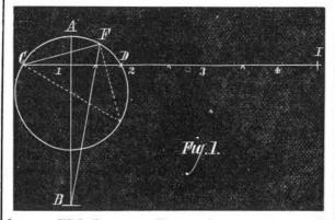
figures. With the same radius, on A as a center, cut the circle in C and D. Draw C D, and produce it to E, making CE, equal to three times CD. Divide CE into as many equal
