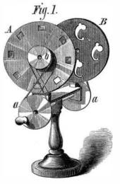
colored image will be produced by each one as it passes, and this image will remain on the retina, by persistence of vision, long enough to make the design appear multiplied symmetrically about the center with great brilliancy of colors. If now the figures, of which the design consists, are made to change successively in form and position, as in Plateau's phenakistoscope, the surprising effects of the graceful motions of the images in that apparatus will be combined with a splendid coloration.
