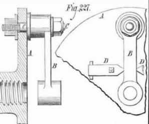
from moving sideways during the operation of boring. Th use of this stud, modified in shape to suit the work, is als applied to the turning of cranks, eccentrics, and other similar work, requiring unusual exactitude in the position of a hole or holes, or of a diameter in its position relative to a hole.
