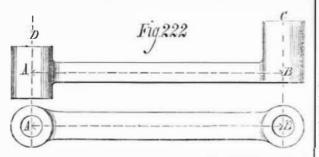
hightof the surfaces upon which our circles are to be marked from the body of the lever or arm. If the arm is to be finished along its whole length, it is better to mark off the body of the arm first, which we perform as shown in Fig. 223. Setting our work upon the table, A, and wedging it as shown, we mark off with the scribing block the lines, C C
