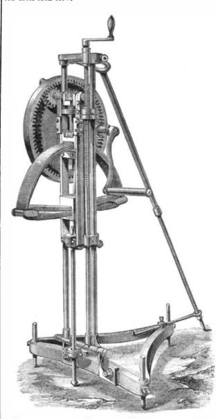
The tool is struck rapidly by a steel-faced hammer worked by a crank through the medium of a spring. The throw of the crank is 1½ inches; but when in full work the hammer, under the action of the spring, moves about double the stroke due to this throw, a speed of 40 revolutions per minute of the handle causing 212 blows per minute of about 5 inches fall to be struck by the hammer. The machine was awarded a prize at the recent exhibition at Manchester.
