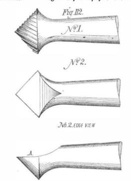
serrations forming cutting edges or teeth, and No. 2 is filled at the conical end exactly to half a diameter, the edge, A, performing the cutting. Either of them will cut true and smoothly, oil being applied when they are used upon steel or wrought iron.
