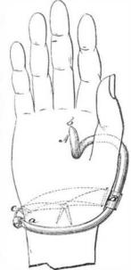
hand, the husker being attached to the other hand in the manner above mentioned; the corn is thrust through the husks, stripping the husk from the ear in a rapid manner and without injury.
