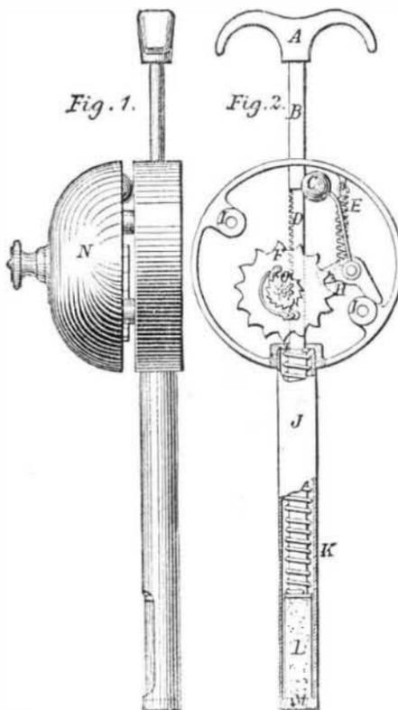
drop by drop through the hole, M. As this melting takes place, the spring, K, forces down the spindle, B, and in so doing gives motion by the rack, D, to the pinion, G, and thence by the ratchet, O, to the striking wheel, F. This wheel, as it revolves, operates upon the pallet, H, and alternately draws back and releases the hammer, C, which, when released, is made to strike the interior of the bell, N, by the action of the spring, F.
