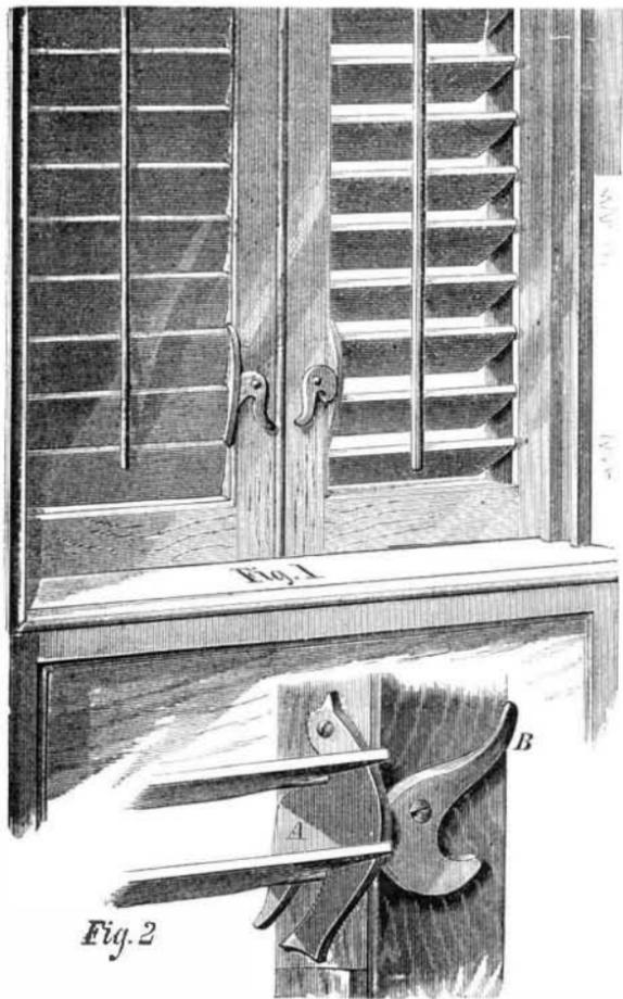
The invention, which is shown attached to the blinds in Fig. 1, and enlarged in Fig. 2, consists of a plate of metal, A, fastened to the stile, and between the latter and the slats, by means of a single screw at its upper extremity. This screw holds it loosely so that it may easily be pushed outward and jammed against the edges of the slats by the cam button, B, after said slats are adjusted as desired. The slats are thus firmly held and cannot be moved or opened from the outside.
