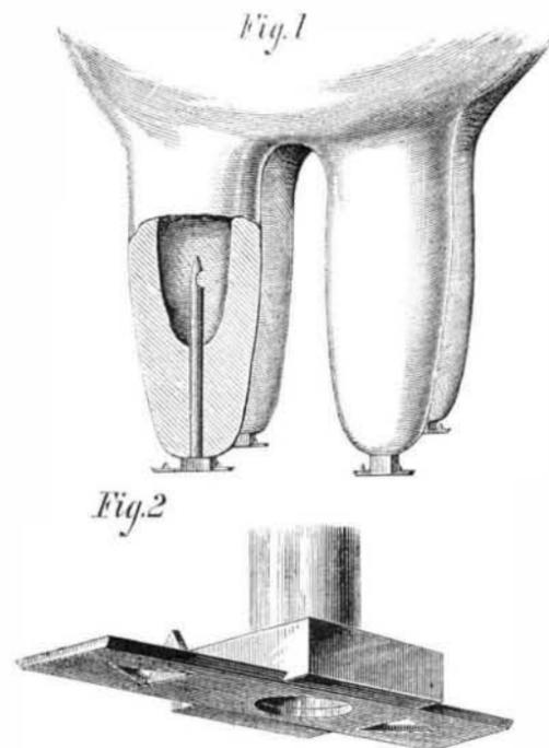
greater rapidity, since the usual squeezing process by the hands is done away with, and to extract every drop of milk which may be contained in the udder. The tubes are neatly made of German silver.
