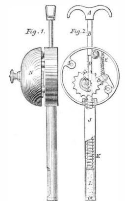
drop by drop through the hole, M. As this melting takes place, the spring, K, forces down the spindle, B, and in so doing gives motion by the rack, D, to the pinion, G, and thence by the ratchet, O, to the striking wheel, F. This wheel, as it revolves, operates upon the pallet. H, and alternately draws back and releases the hammer, C, which, when released, is made to strike the interior of the bell, N, by the action of the spring, F.
