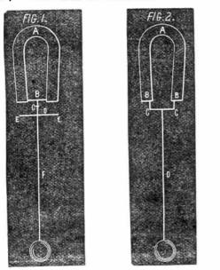
However, as pendulums left free to vibrate make a revolution in direction in twenty-four hours, it is possible that, when vibrating from side to side, the magnet would hold the crossbar, etc. This would be obviated in part by making the armature, E E, of a circular plate, and would be entirely so by using the following arrangement:
