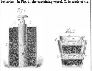
into which a rod of zinc, Z, wrapped in canvas, shown at B, is placed. The space between the tin and zinc is then tightly packed with small pieces of hardwood charcoal, C. These cells are charged with a strong solution of potash made in hot water. In making up this battery, the zinc of one cell is connected with the tin of the next. This battery should be placed on an insulating substance.
