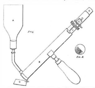
the glass disks come in contact with each other. Through an opening, near the upper end of the smaller tube, is inserted one end of a rhombic prism, E, in which total internal reflection takes place twice. This prism extends halfway across the inner tube, so that an eye, looking through the eyepiece, sees the field of vision nearly half filled by the surface of the prism (see Fig. 2).
