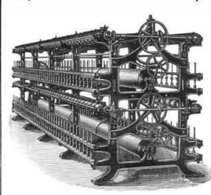
bobbins, after which the bobbins are taken to the doubling rooms, and there the silk from two, three, or four spools is wound together upon one. Finally the silk is spun, and this is done upon spinning frames of two or three stories and containing hundreds of spindles which revolve at a very high velocity.
