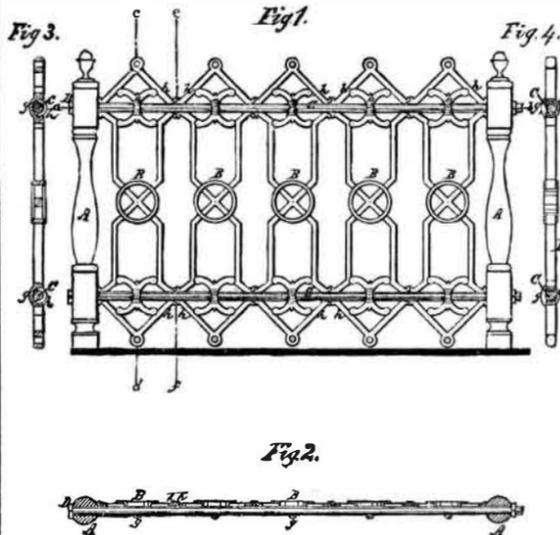
With sections thus cast, all that is required to make a panel of fence is to pass rods or gas pipes through a sufficient number of sections and the posts, and then bind the whole together by screwing nuts on the ends of the tie rods, when the panel is ready to be erected. Where large hollow posts are used the nuts may be concealed in their interiors.
