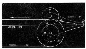
ner: The line is to be placed between two griping rollers, C and D, which are pivoted on a frame, A, and passed into a guide hole, B. The rope to establish permanent communication is passed over a griping sheave, E, which is made fast to one of the rollers, and revolves with it on the same pivot, and is of a larger diameter than the rollers. On revolving the sheave by means of the rope, the whole can be made to travel in either direction. B. FRESE.
