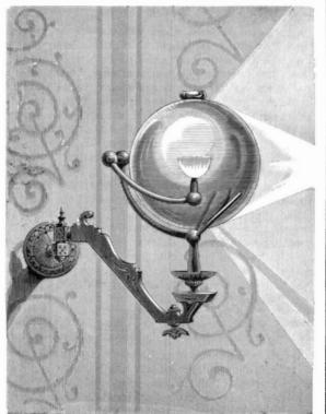
lens and adjustable bracket. The lens is hollow and is filled with filtered water or a solution of salts; its diameter, for general purposes, is about six inches. The bracket consists of an ordinary ground burner and socket, the latter joined to the adjustable or swinging arm. The lens is supported at three points, namely, by the lower or stationary half of the swinging arm and by two small supports projecting from the upper part of the socket.
