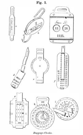
departure and destination. i is a metallic disk with radial slots and corresponding numbers. The strap is so rove through the slots as to give the required indication. The
