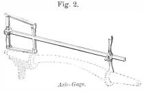
2 shows a gage in which the concave end of the sliding gage is placed on one spindle and the other spindle is set by adjustable bars. The
