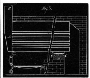
average value for the proper area over bridge wall is three twentieths of the area of the grates; and though in practice this area is very differently adjusted by different masons, the best results are obtained when the area is an approximation to the figure given above.
