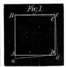
pose the workman starts on a straight edge, A B, and applies his square at B, laying off what he thinks to be a right angle; but partly from the error in the line, and partly from want of accuracy in working to the line, he actually makes the angle at the corner, B, A B c, which exceeds a right angle by the angle, c B C. Proceeding to the corner, c, he works
