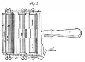
The engraving represents the device ready for printing in blue, red, and green, and showing the other rollers lifted out of connection with the type. When it is desired to print in black or any single color, it will be necessary to use a single roller, as G or H, and raise all the others off the type cylinderinto their respective rests, F. The rollers are wrapped with flannel or its equivalent, so as to absorb a sufficient amount of coloring material to feed the type uniformly.
