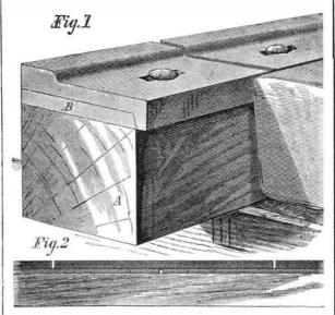
It is also claimed that the compound rail is stronger than a solid rail of the same thickness, and that, as it has no battering or bending points, the jarring so destructive both to rails and rolling stock is avoided.
