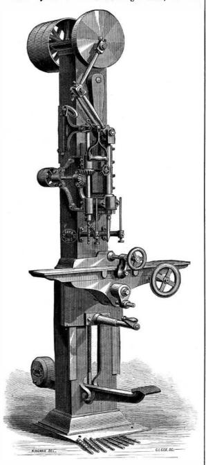
cally reciprocated chisel has obtained a preference. Other systems, such as rotating tools of various designs, are in use for special purposes where the same results could not be produced, or the stuff be conveniently handled, with the reciprocating mortising machine.
