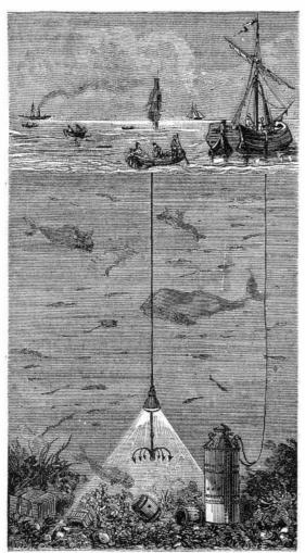
bell and closed the lid, he descends by allowing the water to enter the lower part of the cylinder, and he can come to the surface by ejecting the water by means of a pump placed inside the bell. Thus no rope or tackle is used, and the only necessary connection between the bell and the attendant boat s a telegraphic wire, shown in our engraving
