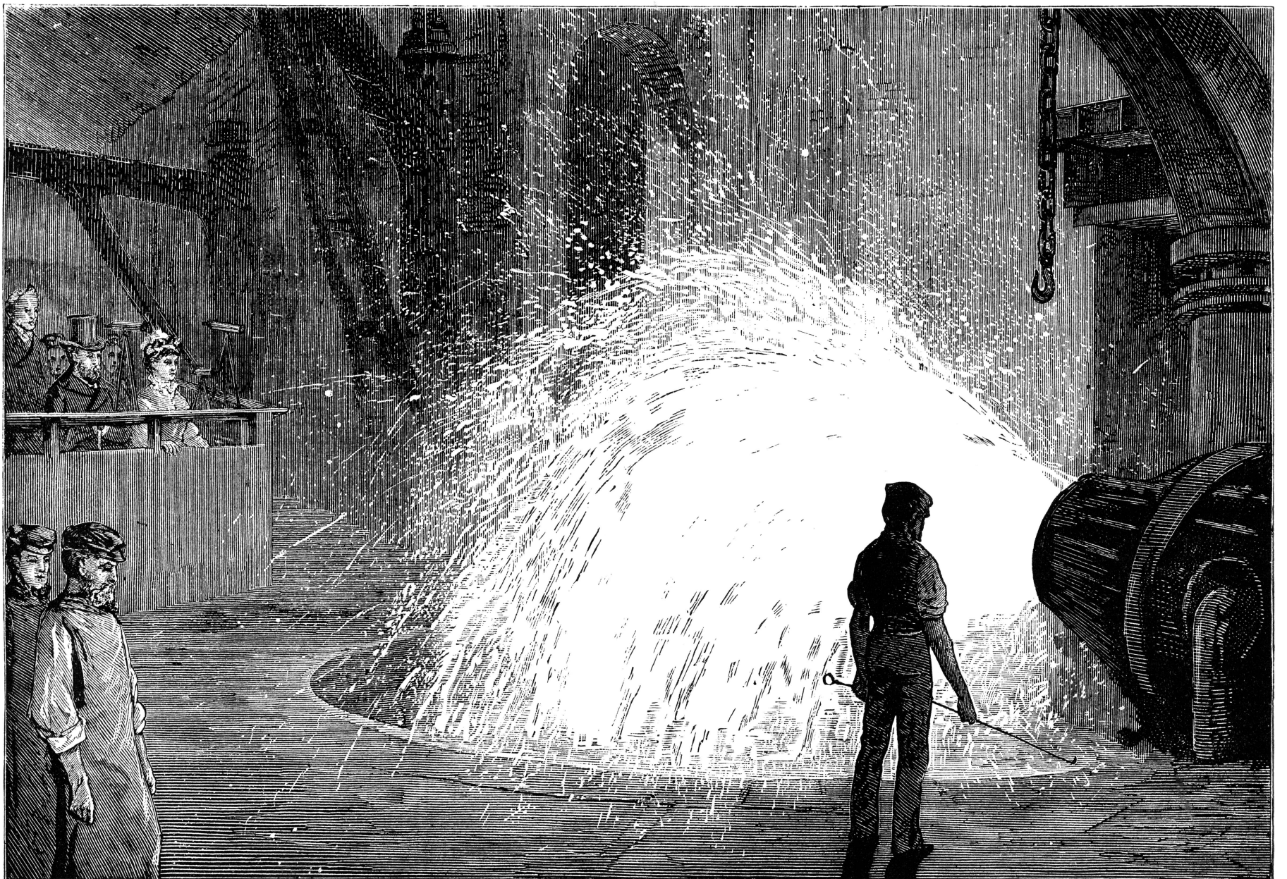
THE BESSEMER STEEL PROCESS.—EMPTYING A CONVERTER
