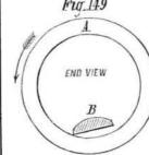
places of a hole that is oval, or the small end of one that is taper and requires to be made parallel. The smoothness of its work is much improved by smoothing its edge upon an oilstone. Here it may be well to state that the application of an oilstone to the cutting edges of a boring tool increases its tendency to chatter; if, therefore, a hole requires to be made unusually smooth, the tool must be given less top rake and may then be oilstoned. In many cases a tool may be
